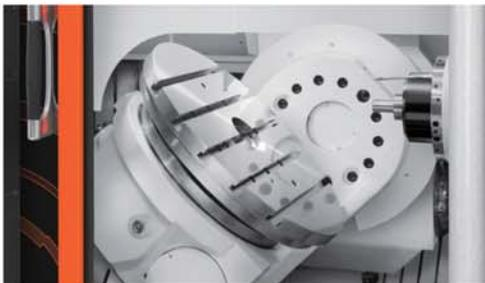
**Simultaneous 5-axis horizontal machining center for high speed machining of aluminium**
