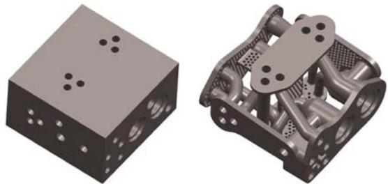
Fuel Manifold re-designed by CYIENT engineers to achieve 42 percent flow performance improvement and 70 percent reduction in weight. Left: Original Fuel Manifold. Right: Fuel Manifold designed for Additive Manufacturing. Original model courtesy: GrabCAD
