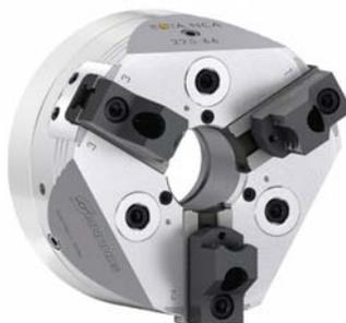
from being lost gradually. Compared to conventional power lathe chucks, the lubrication intervals are extended by a factor of twenty. In addition, the seal prevents chips or dirt from penetrating the chuck body. To ensure maximum process reliability, all functional components are hardened and ground. The fine-serrated power lathe chuck (1.5 mm x 60° or 1/16" x 90°) is available in five sizes from 160 mm to 330 mm diameter with maximum clamping
