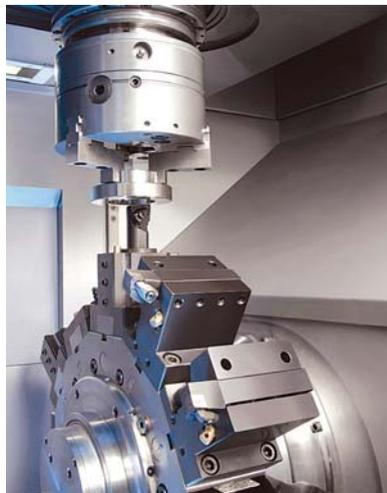
**Machining area of the VL 2: 12 turning or up to 12 driven drilling and milling tools ensure that a variety of machining operations can be carried out in a single setup. The machine can be equipped with a Y-axis as an option.**
