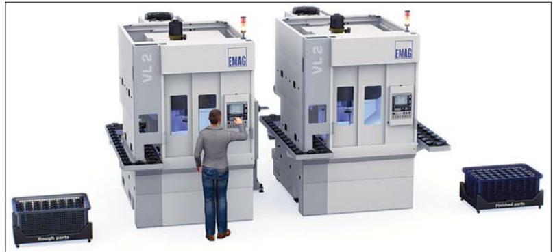
**VL 2 manufacturing system for chucked components.**
