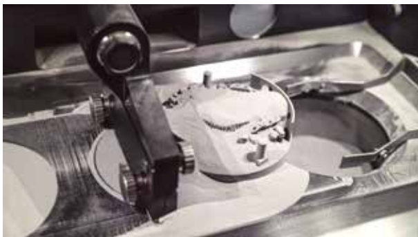
Equipped with Multiplate, the TruPrint 1000 3D printer's recoater pushes the substrate plate into the overflow container after printing. (Source: TRUMPF)
