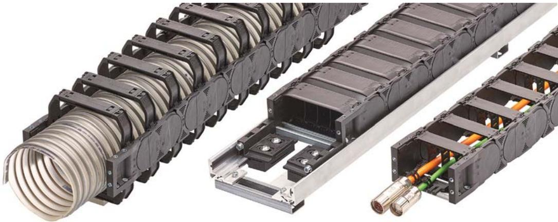
Due to the modular design, the E4.1L energy chain can be adapted to any specific application. As an open standard version for cable routing, with brackets for hoses, or enclosed in a chip-resistant tube in a guide trough – just three of many customising options. (Source: igus GmbH)
