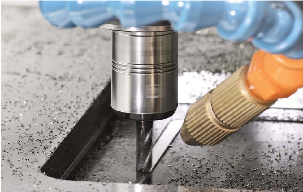
In mold making, the combination of ultra-precision machining centers and SCHUNK TRIBOS polygonal toolholders achieve perfect surfaces.
