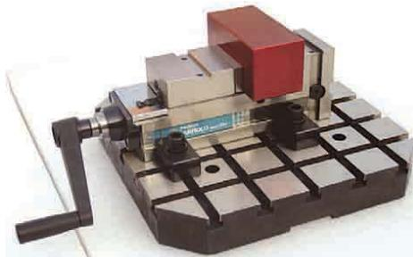
force at different intervals. Thus enables to clamp rigid components at high pressure and slender components at accurate and lighter pressures.
