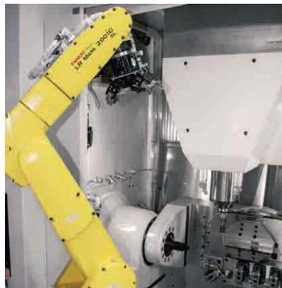
Thanks to variable programming and suitable devices, different parts can be automatically milled without set-up operation.
