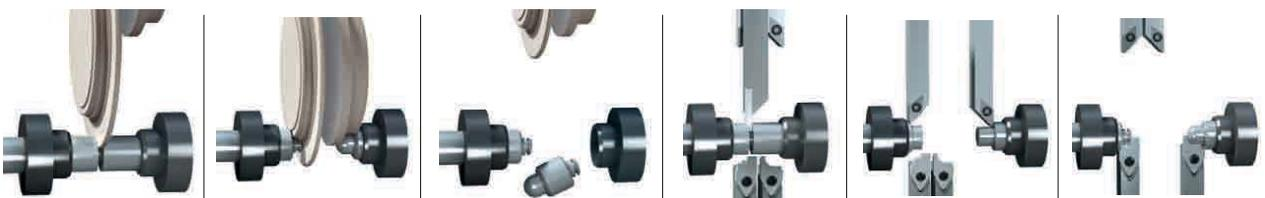
Lightening speed process: The high-speed grinding process has long since finished the job, while the lathe is still working away.
