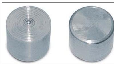
**Left: The lathe leaves a residual cut-off burr in the center of the workpiece.**
