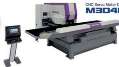
CNC Servo Motor Driven Ram Turret Punch Press
