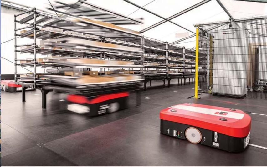
**Driverless transport systems supply parts autonomously**
