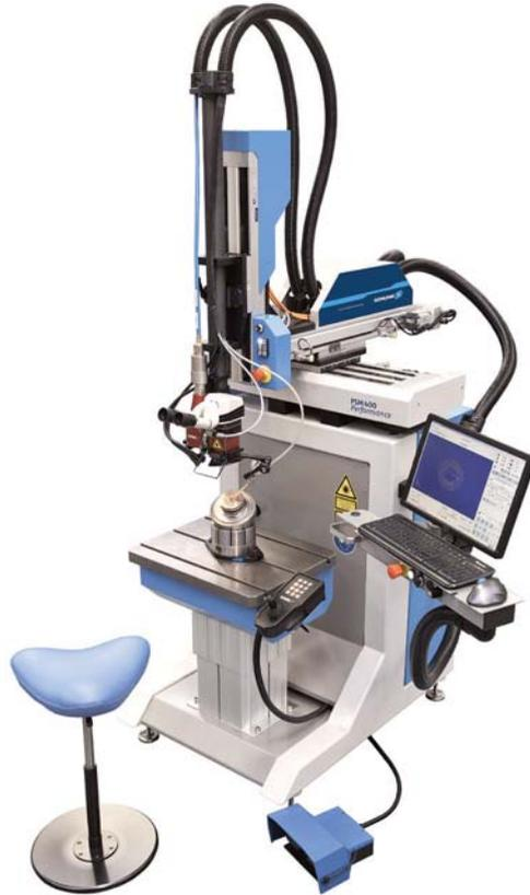
The economically priced PSM 400 Performance from SCHUNK Laser Technology is designed specifically for laser machining in tool and die construction.
