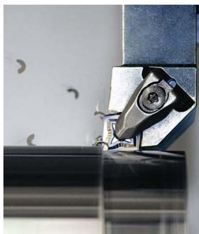
The SF and SM geometries support turning of difficult to machine materials.
