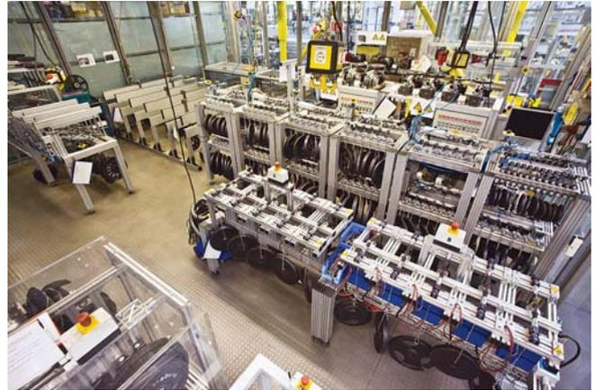
igus tests the abrasion resistance of 3D print filament iglidur J260 in comparison with ABS and injection-molded parts in their test laboratory. (Source: igus GmbH)
