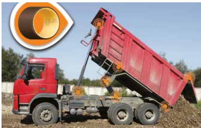
less grease and oil escapes into the environment, a result of which the annual consumption of over 35 million metric tons of lubricant, as measured by RWTH Aachen University, is reduced. Another advantage: the injection-moulding method used to manufacture the plain bearings is especially cost-efficient.
