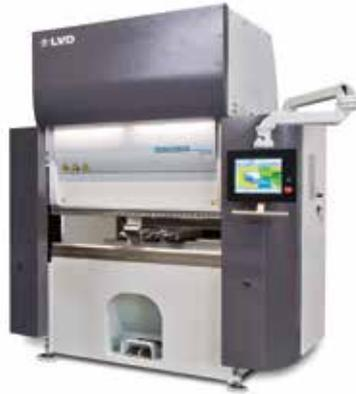
and the servomotors is made using two heavy-duty ball screws to distribute force and tonnage evenly across the working length. As a result, the press brake provides fast, energy-efficient operation across a range of bending jobs.
