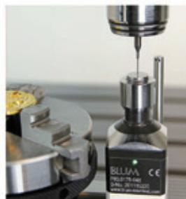
**Z-PICO** – Tool Seeting probe for drilling bit breakage detection and length measurement in micro-machining
