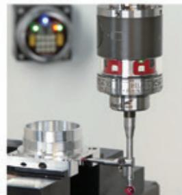
**TC54 -10 | TC64 -10** – Compact touch probes for turning and milling machines
