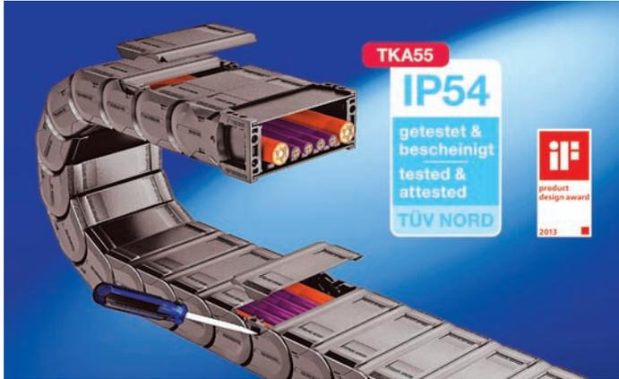
mechanical stresses, e.g. when used with hydraulic lines. The smooth, dirt-repellent contour of the sidebands with their encapsulated stroke system prevents the entry of any foreign objects. The TKA55 cable carriers are particularly tight and therefore reliably protect cables and hoses from dust, dirt, chips and spray water right up to the connection area in accordance with protection class IP54.
