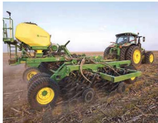
The first thing customers will notice on the N500C is the main frame and commodity tank have changed, with the blower mounted in the forward position and a raised platform, to give operators easier meter access to clear blockages
