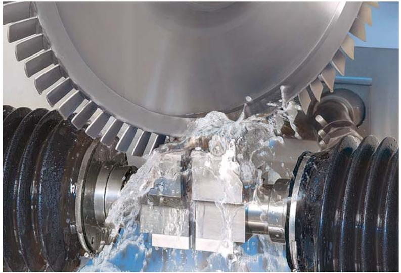
Machining area of an EMAG PO 900 BF for blisk machining using PECM (precise electro-chemical machining) technology
