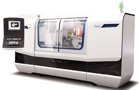
Proven S33 features: Unique arrangement of the motor spindles. Very simple changeover from grinding between centers to live spindle grinding. Swivelling machine table. Optional C-axis for form and thread grinding. Granitan® machine bed. Large selection of options and accessories.
