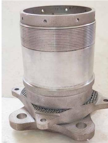
**3D printed rear wheel hub after undergoing post-processing**
