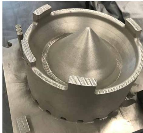
**Additively manufactured, cobalt-chrome sump cover for F110 engine. Produced on a GE Additive Concept Laser M2 machine at the GE Additive Technology Center in Cincinnati, as part of collaboration with the US Air Force's Rapid Sustainment Office (RSO). (Photo: GE Additive)**
