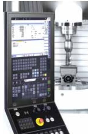
standard. The system guides the user step by step through operation, adapting its interface depending on the task and the context. If required, the full machine documentation and the maintenance instructions can also be called up on the 24" panel. This means that folders and paper are things of the past. TouchLine can be operated intuitively and interactively with the same familiar motions as for smartphones and tablets:
