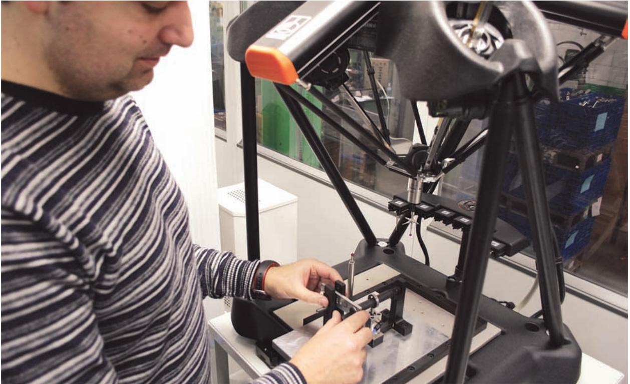
An Eponsa engineer loads a wiper mechanism part onto Equator ready for gauging
