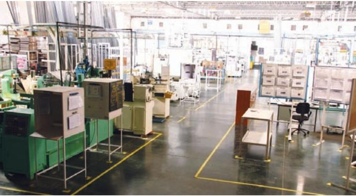
The layout has been designed through value stream mapping and with an aim to achieve the best floor space utilisation
