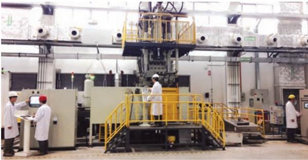
The GM China Advanced Technical Centre (ATC) in Shanghai has started the operation of its Vertical Squeeze Casting (VSC) machine. This is the first in the world designed for developing next-generation magnesium castings. This achievement marks a breakthrough in lightweight materials research by General Motors.
