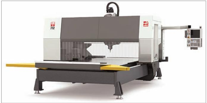
is offered as standard. Fitted with a direct speed belt drive, the routers are capable of generating 23 Nm of torque at 4600 rpm, along with 20.3 m/min cutting feed rates. Also featured are a 10-pocket automatic tool changer (ATC), memory lock key-switch, 15" colour LCD monitor and USB port. Standard G-code programming is facilitated through the user-friendly, full-function Haas CNC control.
