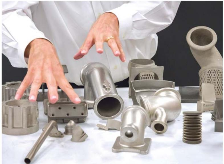
**“3D printing allows design engineers to produce prototypes of metal parts before actually making the final version of them.”**
