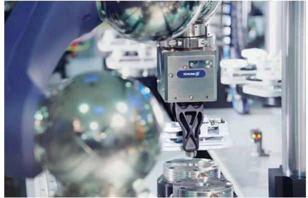
spring assembly. The system is self-locking and designed for form-fit clamping. A system pressure of 6 bar is sufficient for pneumatic opening of the module. All functional components such as the base body, clamping pins, and clamping slides are made of stainless steel.
