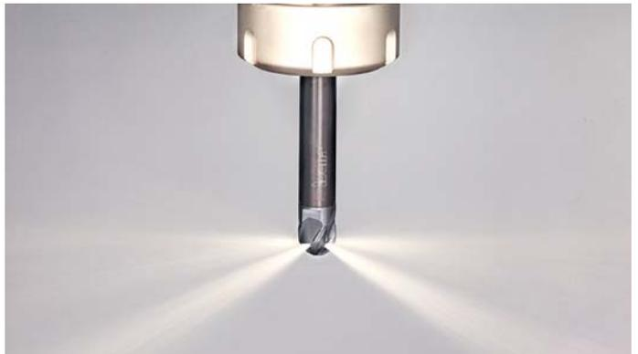
Fig.2 - Multi-Master ball-nose milling head, intended for machining hard-to-cut materials with inner channels for coolant supply in the appropriate area.
