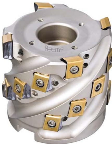
**Fig. 3 - A T490 extended flute cutter intended for HPC. The cutter design enables mounting nozzles in the outlets of the holes for coolant supply.**
