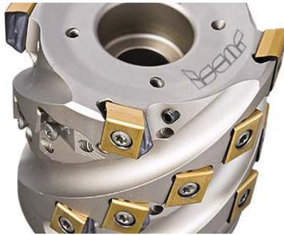
Fig.4 - A nozzle mounted in a hole for coolant supply near a face-cutting insert of the T490 extended flute cutter.
