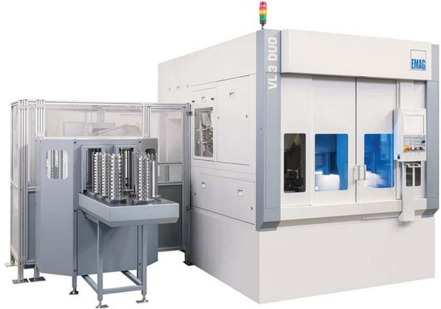
With its range of parts up to 150 mm (5.9 in) in diameter, the VL 3 DUO is ideal for functions in transmission component manufacturing, for instance in the machining of blanks for gear production.
