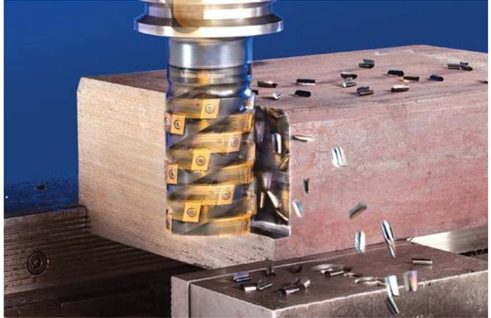
Fig.1 - Wet cooling is not recommended for rough milling steel with the use of a T490 extended flute cutter.
