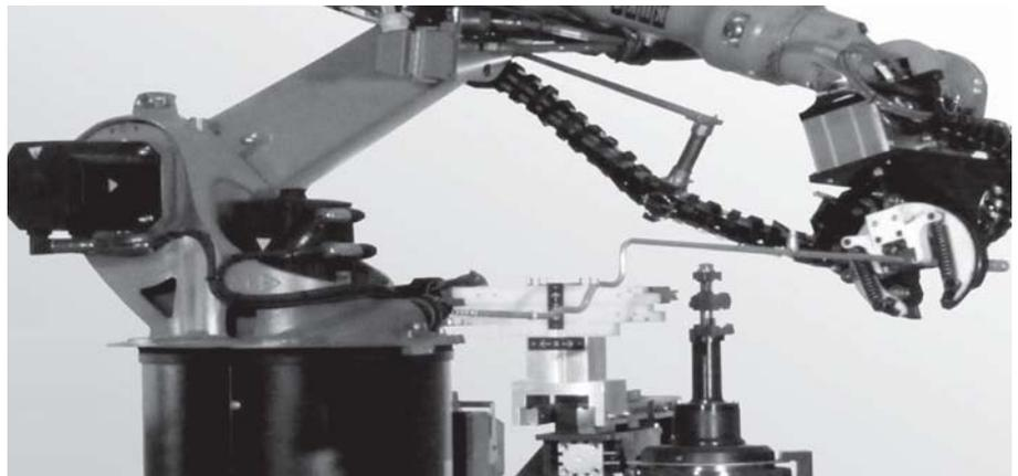
The flexibility and speed of the robot, combined with the patented multi-stack, two-radius bend head, allow the AMT 16 to bend the most complex part shapes (up to 3 different compound bends) in a cycle time faster than conventional mandrel bending.
