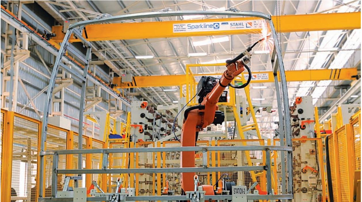
The plant also has robotic welding facilities for main body and under body welding
