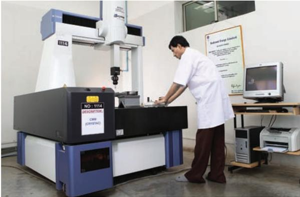
Co-ordinate Measuring Machine for checking critical machining dimensions.
