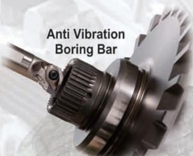
Pin Milling Cutter for Crankshaft Machining
