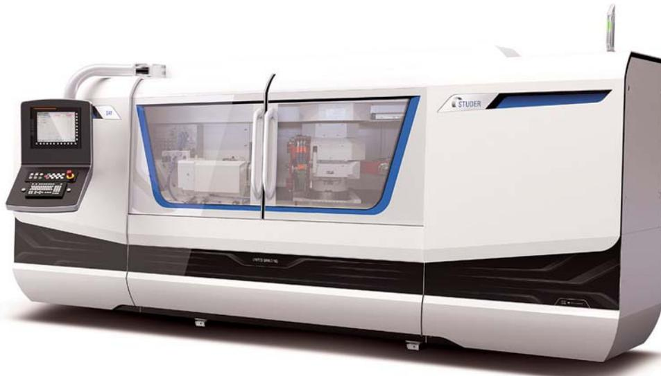
The S41 CNC universal cylindrical grinding machine is characterised by outstanding technology and cost-effectiveness. The machine grinds with much higher precision, paired with a much greater metal removal rate. In addition the longitudinal and cross slide, as well as the swivel axis for the wheelhead are equipped with electric direct drives, which move to the working position much more quickly and precisely.
