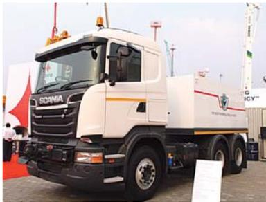
Puller tractor R 580 6x4. According to the certification, Scania R 580 with capacity of gross combination weight (GCW) 200 tons when coupled with multi-axle trailer is now defined under a new category called Puller, and will be now available in the commercial market for our customers. Scania is the first commercial vehicles manufacturer in India to receive this certification from ARAI.
