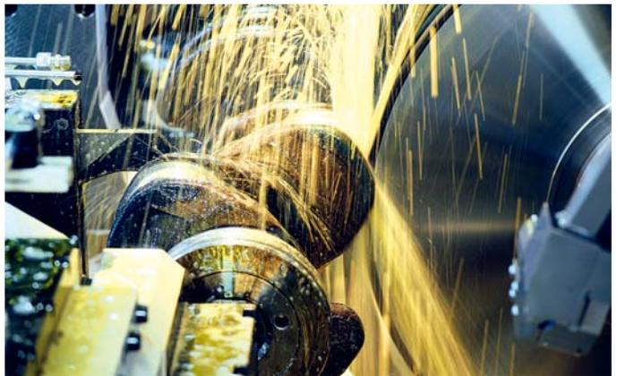
The largest JUNKER platform built to date will soon be put to use for the grinding of crankshafts. Other applications are to follow
