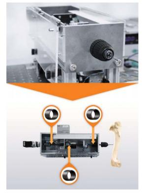
"The combination of rotary drive and axial vibration requires the use of high-quality plain bearings not only to implement freedom of movement in the axial direction, but also to achieve the most accurate signals possible at high vibration frequencies."
