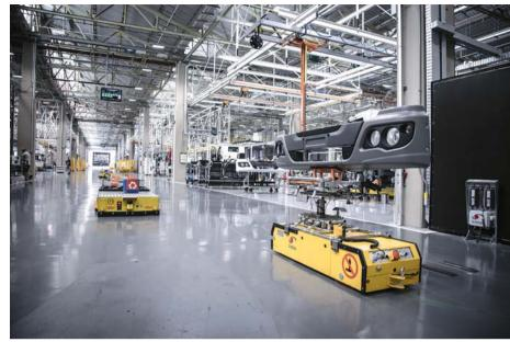
Digitally connected Driverless Transport Systems (DTS) shuttle truck parts to new assembly line at Mercedes-Benz do Brasil's plant in Sao Bernardo do Campo.
