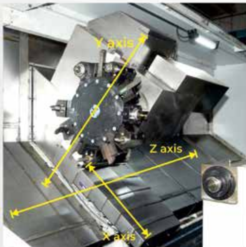
CNC Turning Center 5000 mm Y axis and live tools
