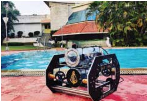
AUV is currently capable of carrying out navigational and other tasks pre-fed into its memory with good precision and near-zero error. Weighing 19.6 Kgs, MEC's Black Pearl is a fully autonomous operation and carries power onboard through a Lithium Polymer Battery.
