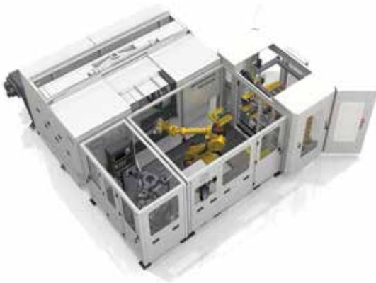
**Pic 3 - Expansion of the shaft machining machines by a "MAG Cell" with automated workpiece measurement and material supply by pallets 10 Simulation and virtual commissioning of shaft machining with the software tools "NX CAM" and "Visual Components".**
