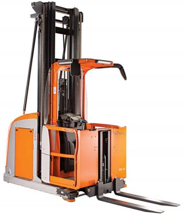
**H**ow are energy and signal cables guided from the mobile hoist frame to the cab of an order picking unit using several guide rollers? The design-engineers for the Still EK-X vertical order picker found the answer: they used a chainflex cable that was originally developed for use in energy chains. Both igus and Still determined from various tests that this cable is not only ideal for applications in energy chains, but will also perform well with guide rollers.
