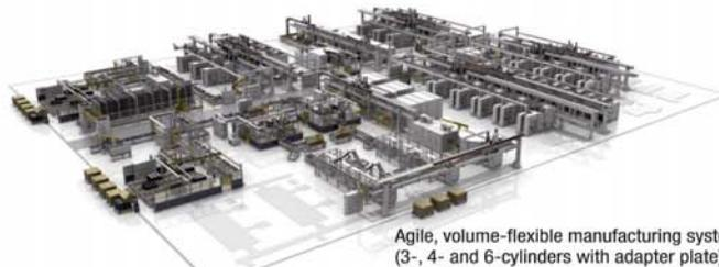
Agile, volume-flexible manufacturing system with adapter plates for cylinder heads (3-, 4- and 6-cylinders with adapter plate) with 32 single-spindle machines (450,000 workpieces p.a.)
