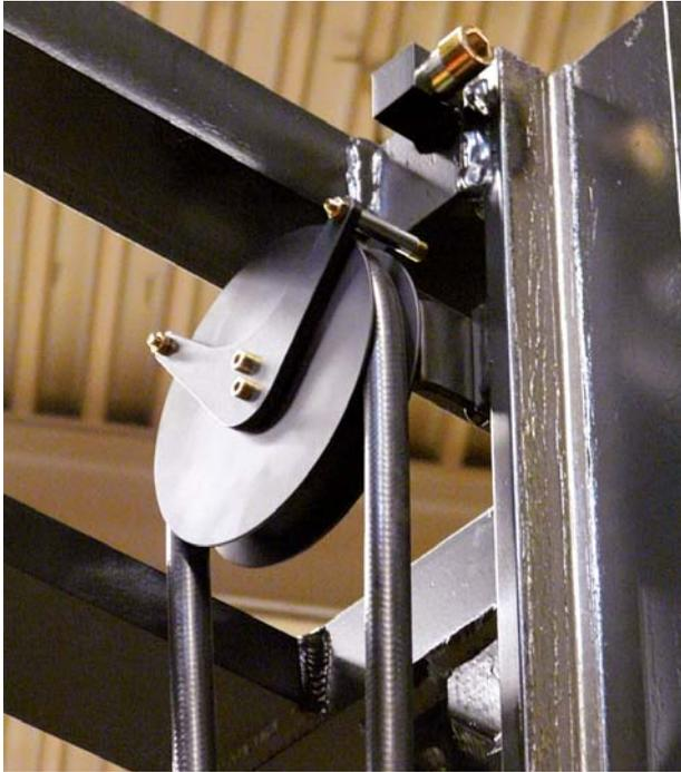
Energy and signal cables up to 14 metres in length are guided in the hoist frame by guide rollers, and move every time the mast is raised or lowered. (Source: igus GmbH)
