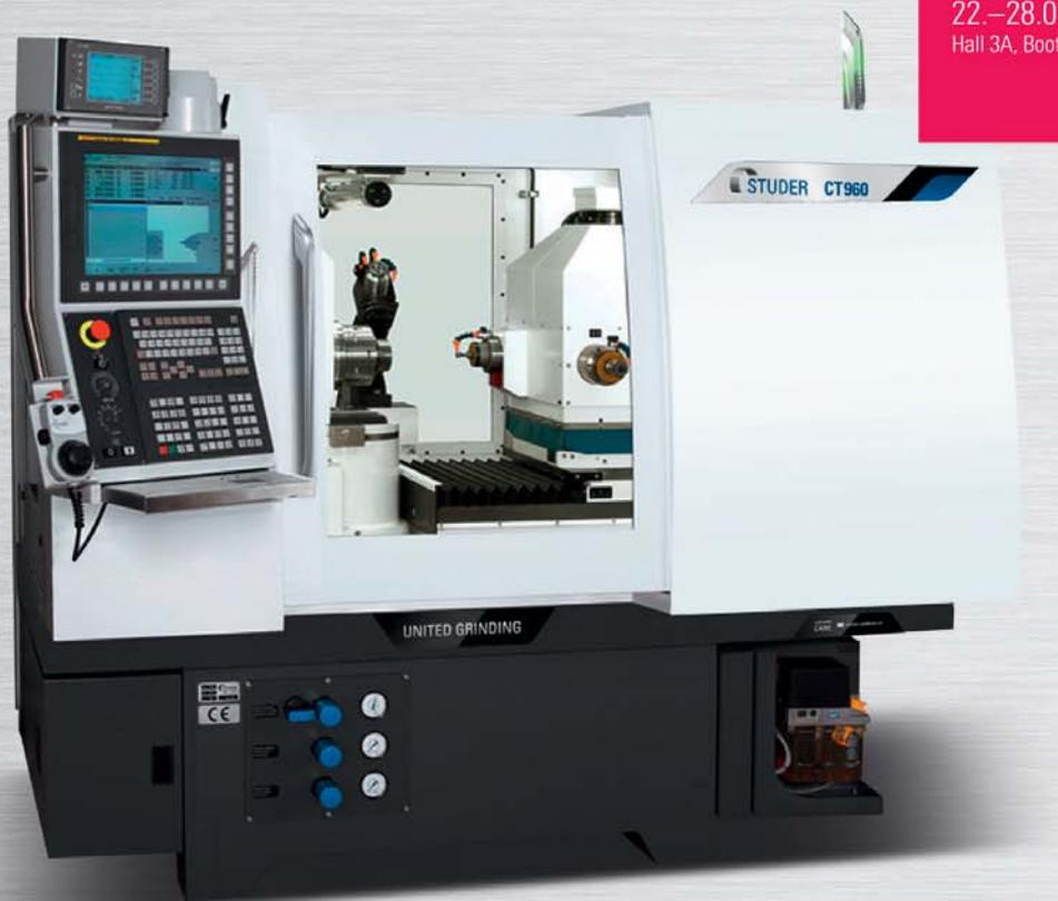
The CT960 with four spindles and a fully interpolating B-axis is a complete universal internal and die profile grinding machine with external grinding options. The StuderSimCT software allows you to program any conceivable internal grinding task in a flash: from radius, through taper to surface grinding. The high-speed axes increase productivity – without compromising on precision.
