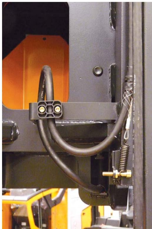
A cable grip ensures that tensile forces are properly transferred to the cable. (Source: igus GmbH)
