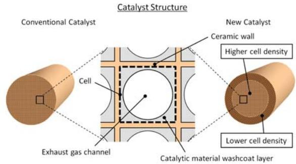
ic precious metals, such as finding the optimal substrate shape and length, as well as modifying the cell wall thickness and cross-sectional area. Other R&D efforts include selectively washcoating precious metals and other catalytic materials, and changing catalytic substrate cell density in line with exhaust gas flows.
