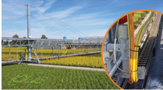
A roller energy chain in a guidelite guide trough ensures safe guidance of the hoses and cables in the precision irrigation carriage.
