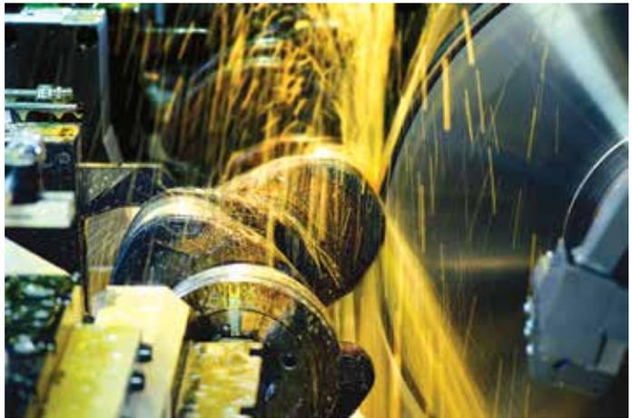
JUCRANK pendulum grinding machines take care of almost every conceivable crankshaft grinding operation.
