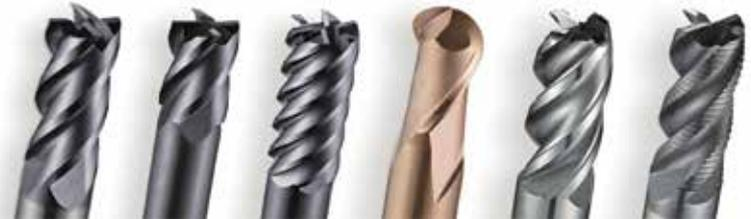
Its differential pitch cutters (S260, S262, S264) reduce chatter and offer fewer tool offset adjustments, providing effective chip removal at high feed rates. The trio of cutters - available in diameters from 3-20mm - feature an optimized cutting-edge to reduce chipping and prolong tool life. All have an AlCrN coating for improved wear and oxidation resistance.
