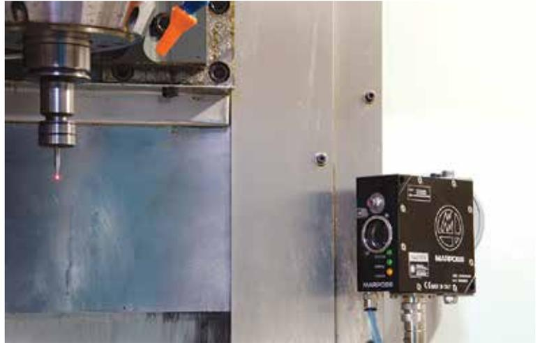
Fast and reliable detection achievable by the TBD allows to reduce production time and to avoid expensive work-pieces scrap due to wrong cutting process by damaged or broken tools.
